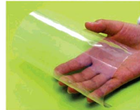
Figure 7. Appearance of optically transparent acetyl BC nanocomposite.
