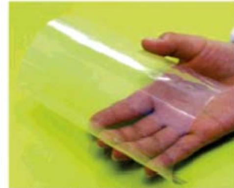
Figure 7. Appearance of optically transparent acetyl BC nanocomposite.
